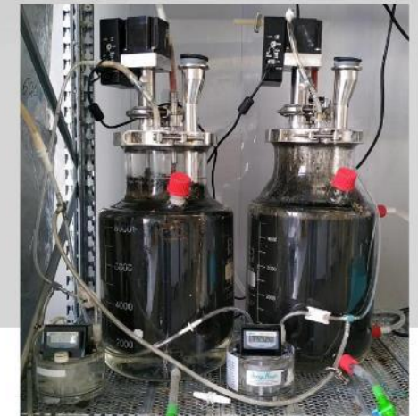
Experimental set-up for lab-scale continuous AD test. Reactor volume 6 liters.
